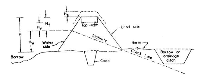
The design height of the levee (H) will be the sum of the design high water storage ( $H_W$ ), the added height ( $H_V$ ) for wave action, if any, and the freeboard ( $H_f$ ). The constructed height will include an allowance for settlement ( $H_S$ ), which will depend on the foundation and material used in construction. The actual design high water stage should be based on the water surface profile.
