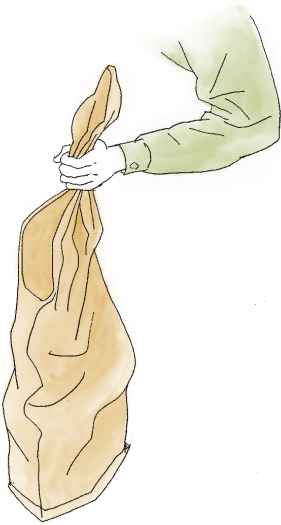
Figure 11A: Sandbag filled 1/4 to 1/3 full
