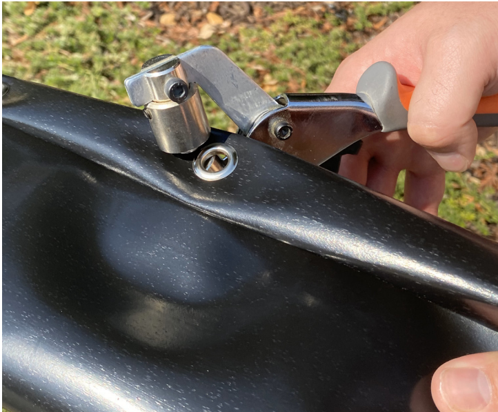
Creating an eyelet using a grommet
