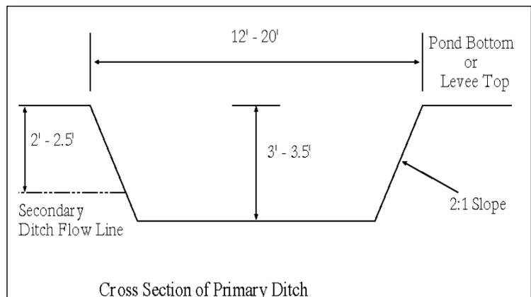
Secondary ditches, usually used on larger properties, supply the pond with enough water to flood up within 10 days, drain within 20 days, and are usually 6-10 feet wide and 2-2.5 feet deep (SRCD 1998). These ditches connect “V” ditches (see below) to primary ditches and ultimately empty out to the water control structure (SRCD 1998).
