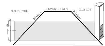
Typical Exterior levee section for a drain gate
