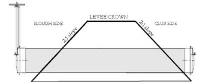
Typical Exterior levee section for a flood gate
