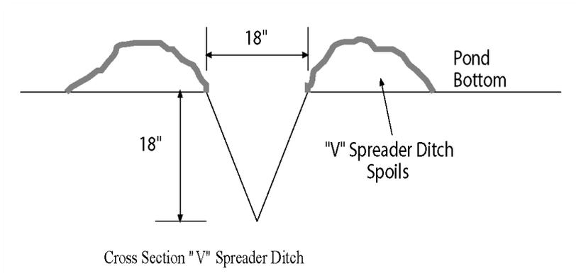
The maintenance of ditches primarily involves removing obstructions caused by vegetation, debris, and siltation. Maintenance is scheduled to maintain the ability to use the ditches to flood and drain the pond in 30 days or less (SRCD 1980).
