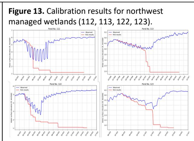
**Figure 13.** Calibration results for northwest managed wetlands (112, 113, 122, 123).
