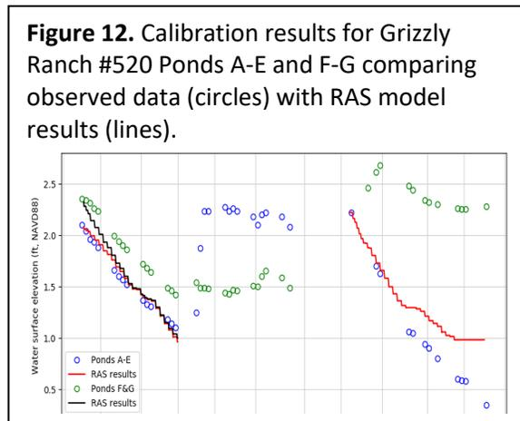
**Figure 12.** Calibration results for Grizzly Ranch #520 Ponds A-E and F-G comparing observed data (circles) with RAS model results (lines).
